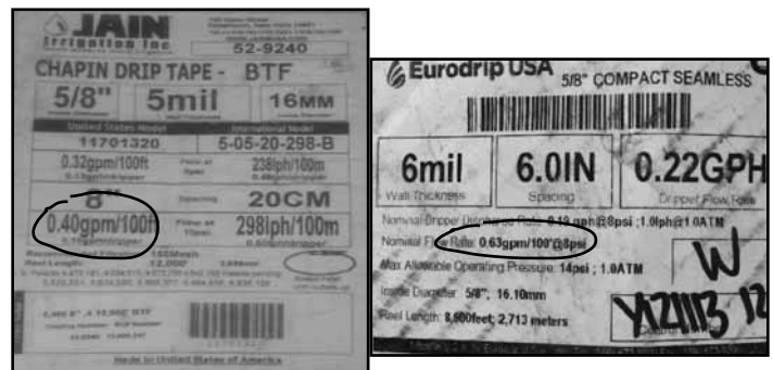
Figure 1: Examples of driptape flowrate from the labels on the rolls
